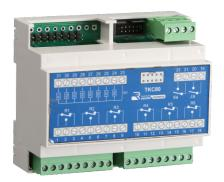
Passive operator module with interface function to power. Equipped with 8 16A relays, it is suitable for driving small loads such as motors, shutters, lamps, medium-power contactors coils, etc. On the front, 8 red LEDs show the individual relays status.
